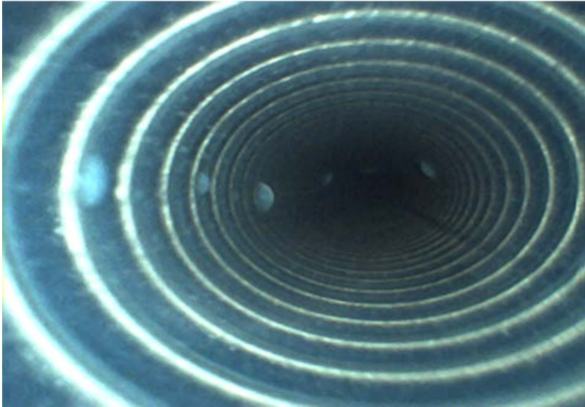
Fluid in Channel of “DRY” scope
